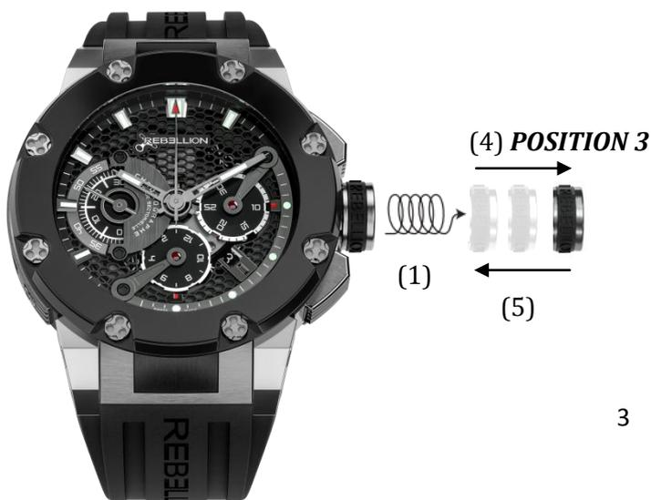
After unscrewing the crown (1), pull the crown out two clicks (4) to **POSITION 3**, adjust the hands to the correct time (NB: around midnight the date will change), simultaneously push and screw the crown back to home position (Details 5-7). When performing this operation make sure that the calendar changes the date at midnight and not at midday.
