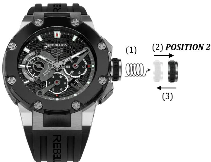
After unscrewing the crown (1), pull the crown out (2) to **POSITION 2** and turn the crown clockwise to set the date. After having set the date, simultaneously push and screw the crown back to the home position (details 3-7). **Please never adjust the date function of your REBELLION watch between 8pm and 3am as it could seriously damage the movement.**
